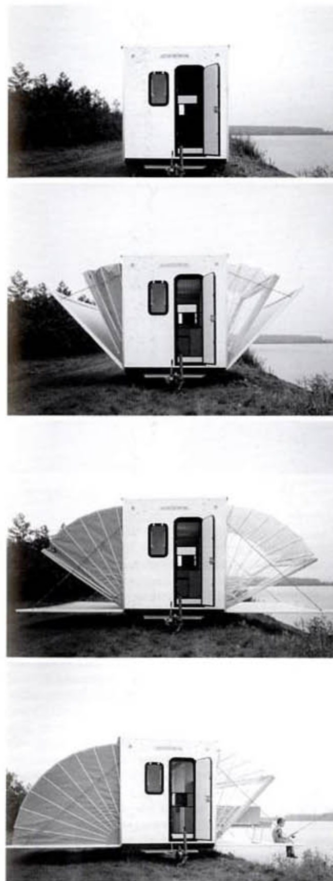
Fig. 11.7 Markies: unfolding sequence (photograph by Roos Aldershoff).
